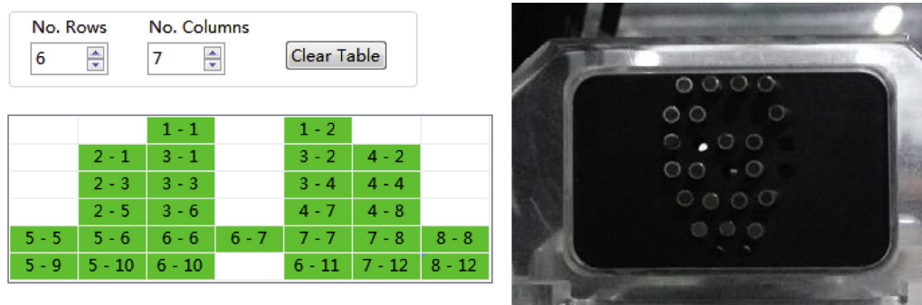
Fig. 1. Sequence of light source and detector. Note: the figure on the right was the data model diagram involving the sequence of light source and detector, the light source (S) was in front of the detector (D). The figure on the left was the physical map of installment of S and D based on the model diagram.
